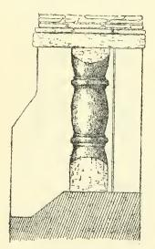
FIG. 114.—Baluster shaft in opening in western wall of Brixworth Church.
