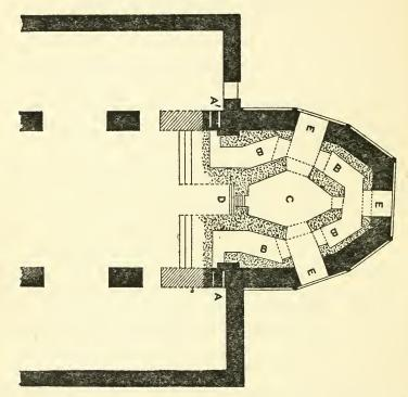
F1G. 160.—Eastern part of Church at Wing, showing the crypt in its relation to the structures above.
