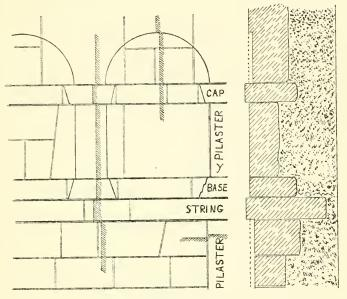
FIG. 76.—Pilasters, arcading, etc., on the exterior of Bradford-on-Avon, with section of chancel wall. Scale  $\frac{1}{32}$  of nature. The original wall face is represented by the face of the upper and lower pilasters and the part above the arcading.
