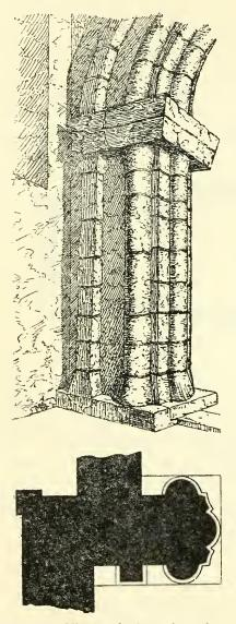
F1G. 59.—View and plan of northern jamb of chancel arch, Wittering, Northants. Scale of plan 1 in. to 1 ft.
