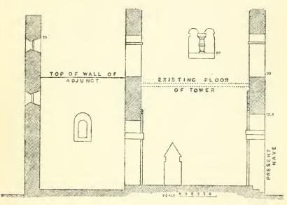
FIG. 130.-Section of tower and western adjunct, Barton-on-Humber.
