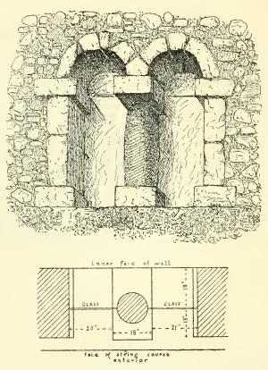
FIG. 39 .- Window in north wall of nave, Worth, Sussex, with plan.
