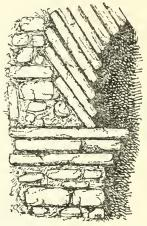
FIG. 150.—Springing of arch at Brixworth.
