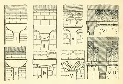
FIG. 26.—Methods of dividing a double opening.
