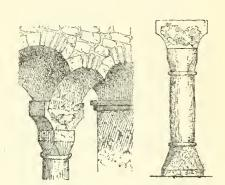
FIG. 115.—Baluster from FIG. 116.—Mid-wall baluster shaft from Wing, Bucks.
