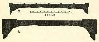
FIG. 35.—Comparison of Saxon pilaster strips at Earls Barton tower (A), with Early Norman corner buttresses at West Malling Church, Kent (B).
