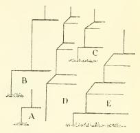
FIG. 31.-Plinths of Anglo-Saxon walls. (Scale, c.  $\frac{1}{2}$  in. to I ft.)
