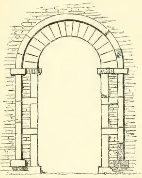
FIG. 48.—Tower arch, Brigstock, Northants, showing pilaster strips carried round the arch. The pilaster strips on each side start from projecting corbels. From a drawing by the late J. T. Irvine.
