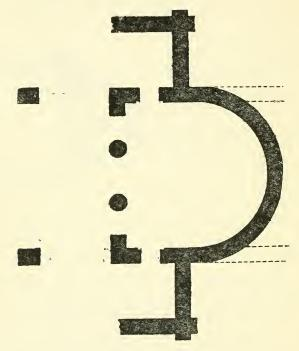
F1G. 155.—Plan of Saxon work at the eastern end of Reculver Church, Kent. From plan by George Dowker, F.G.S.
