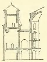
FIG. 21.—Section of western end of the Minster at Aachen. gallery above, but rather with the imposing western forebuilding which contains the entrance portal and serves other purposes presently to be explained. This has been altered in its upper portions in later times but the original form can be recovered, and it seems to have presented the appearance shown in Figs. 20 and 21 which are founded on the restoration published some years ago by C. Rhoen of Aachen.
